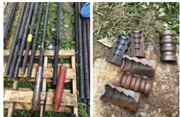
(a) Connector with thread bar (b) Base expansion structure
